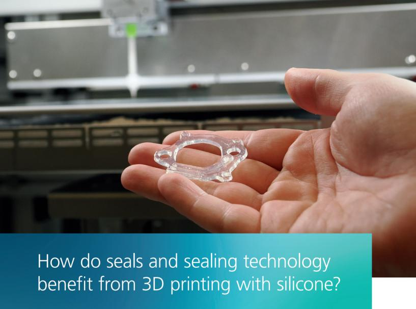
When it comes to custom production of seals in small quantities, such as batch sizes of one or prototypes of new seal geometries, creating the necessary tooling can be very costly.
