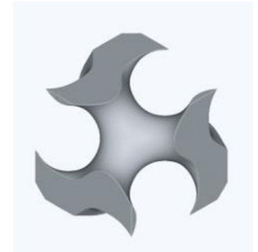
Solid Gyroid Relative density: 20 %
