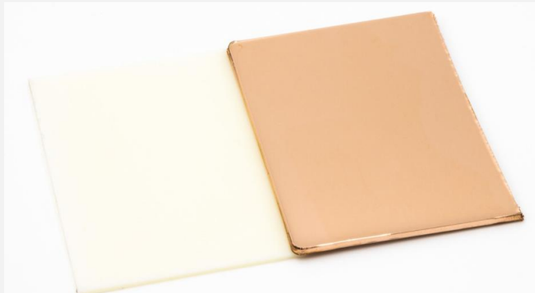
Thermoplastic electrocoated with Cu using a Cr(VI) free pre-treatment step developed at Cidetec
