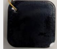
After chemical polishing Ra 3,4 \mu\text{m} Black finishing
