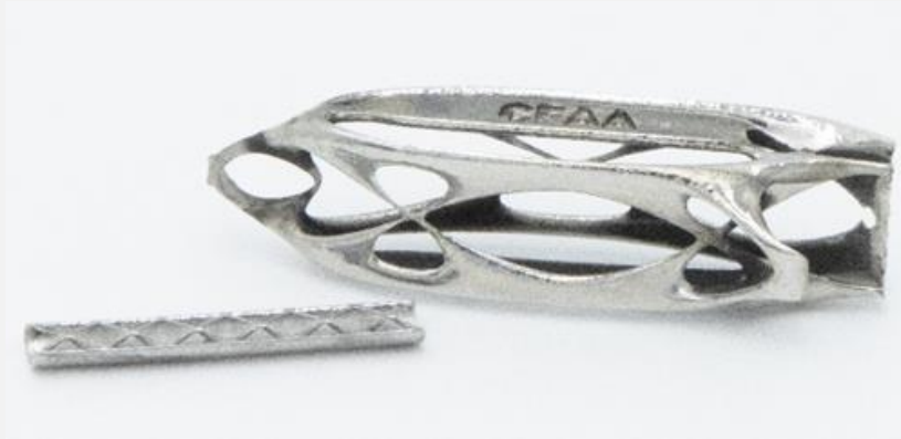
Inconel 718 produced by SLM
