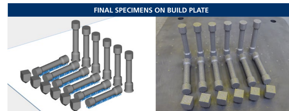
Figure 18: Image of final specimens on the build plate – CAD and image
