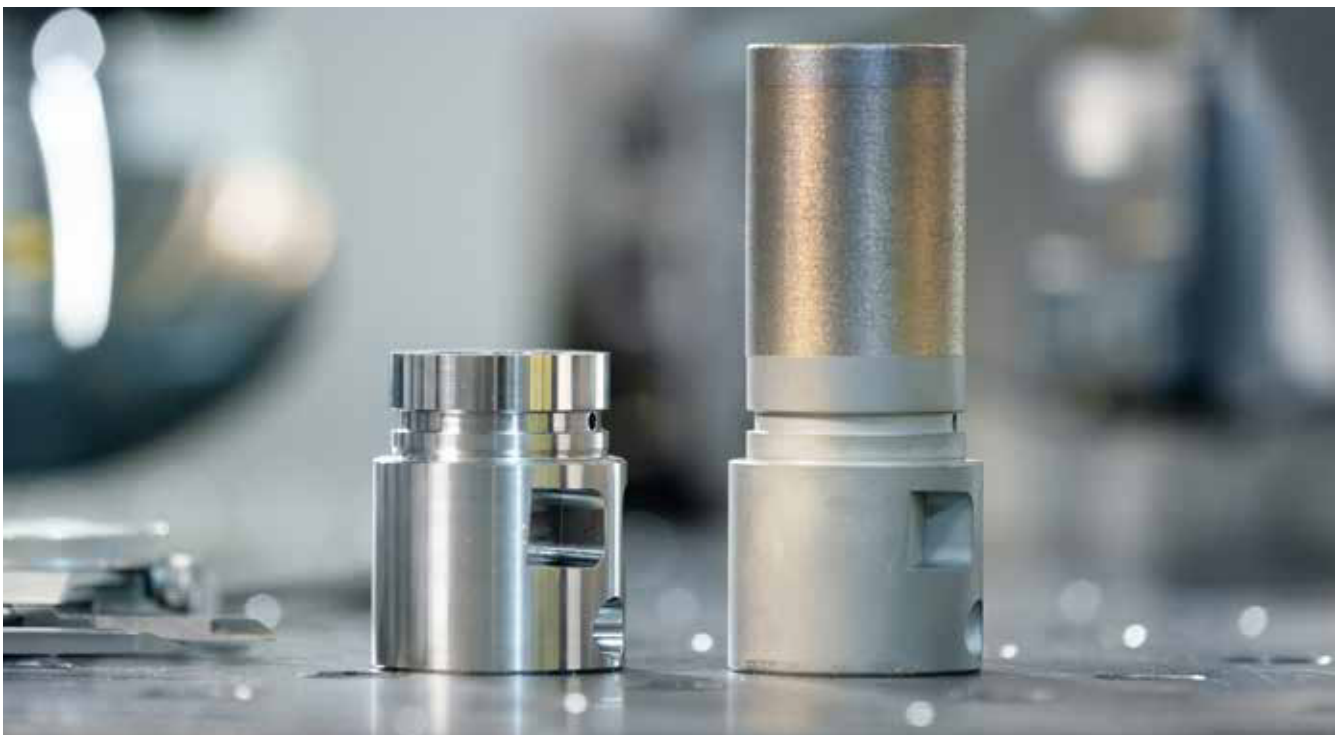
Figure 23: Expansion mandrel, directly printed to a standard base unit, using LPBF technology
