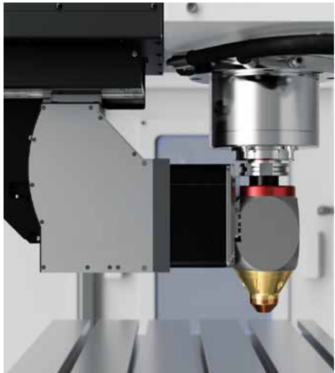
Figure 7: Automated tool change system of a milling machine for a laser metal deposition process head including its supply unit [Hyb22]
