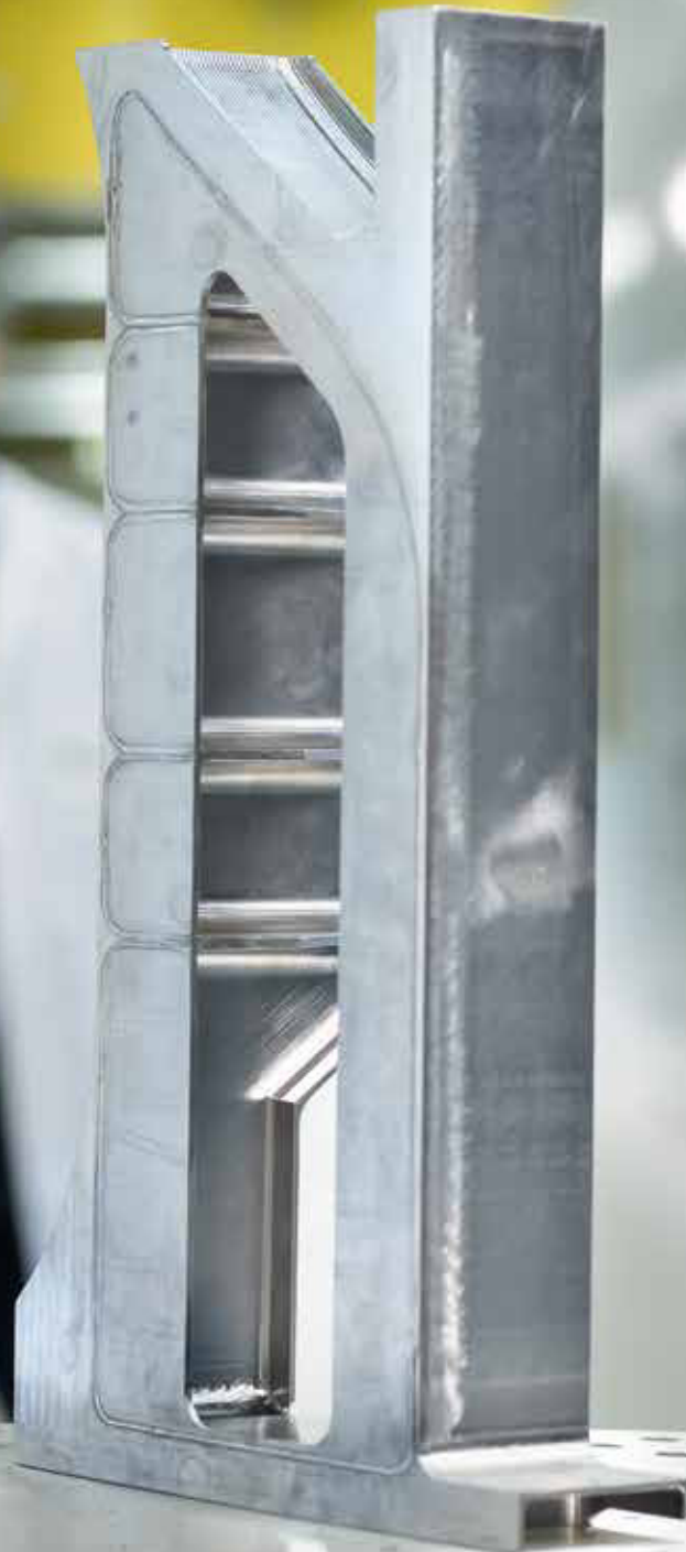
Figure 20: This part of an aircraft door is a use case for manufacturing a hybrid component with welded-in reinforcing plates
