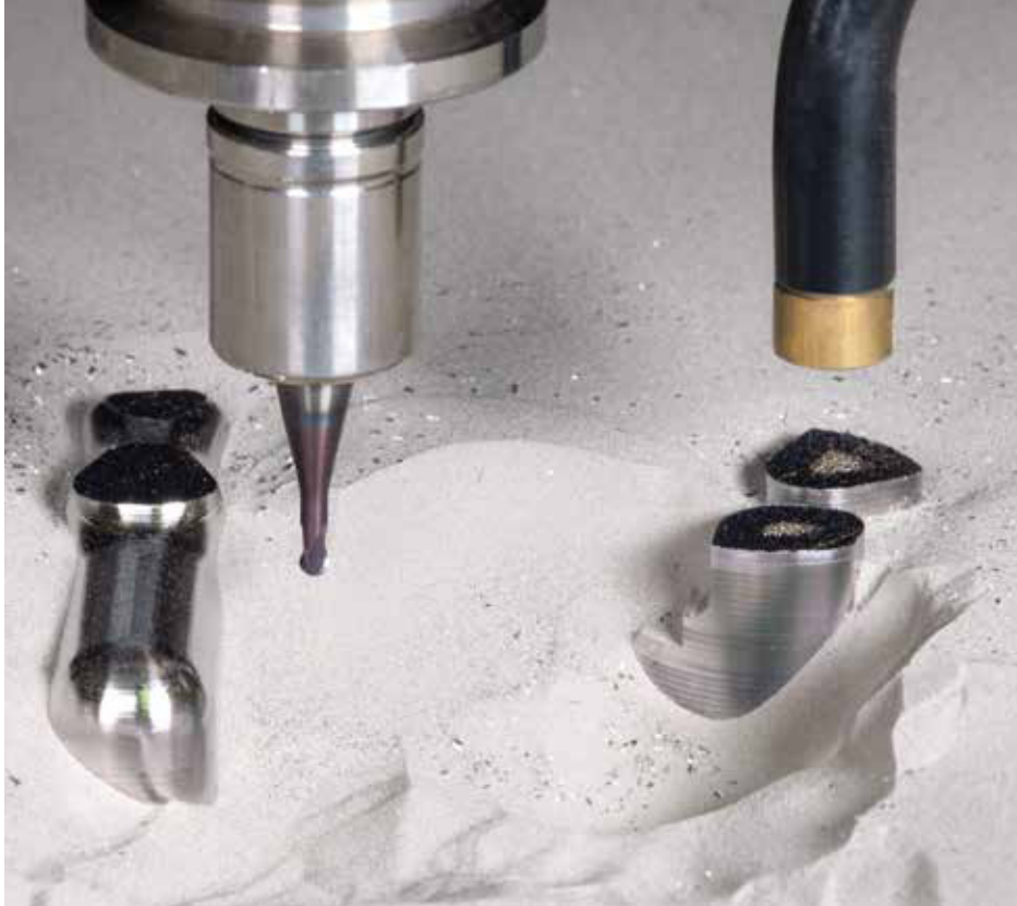
Figure 8: Layer-by-layer milling of the component contour in the LPBF process with an integrated milling head [Mat22]
