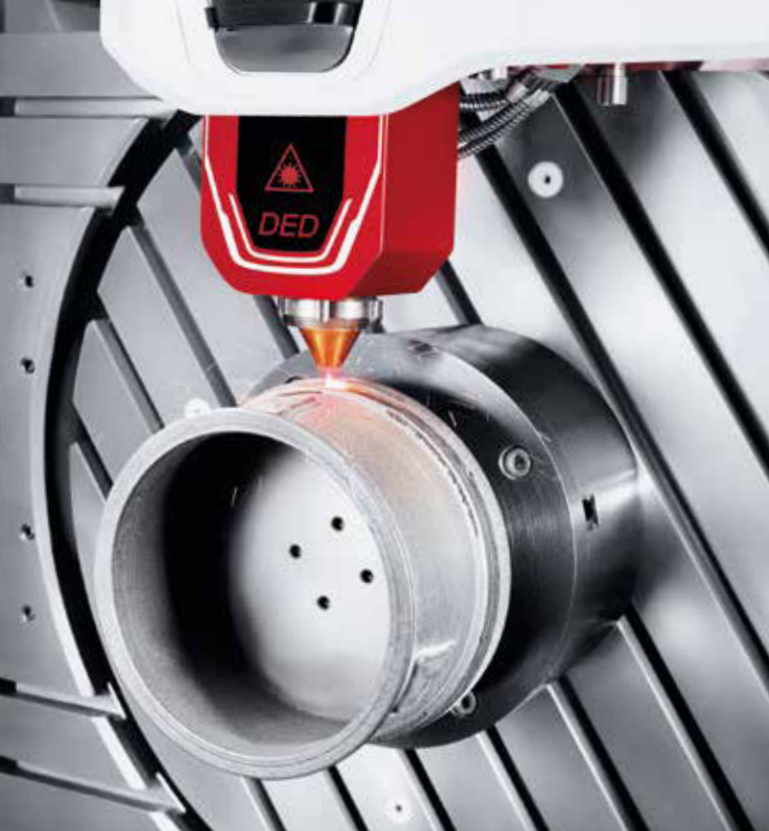
Figure 516: Two processes are combined in one machine to print a net-shape geometry using laser powder deposition and a milling process (either in between or at the end) to machine the part to the final contour [Dmg22]
