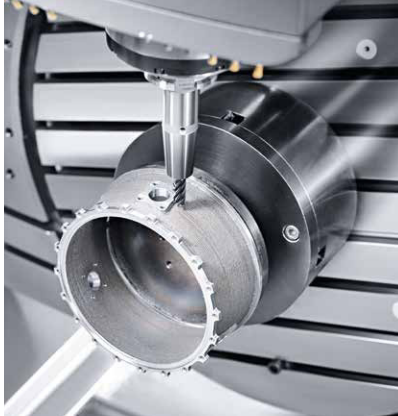
Figure 516: Two processes are combined in one machine to print a net-shape geometry using laser powder deposition and a milling process (either in between or at the end) to machine the part to the final contour [Dmg22]
