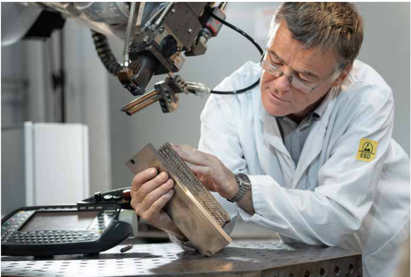
Figure 15: The additive processes are qualified by means of a variety of elementary geometries
