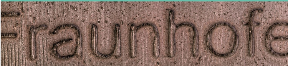
Figure 5: From top to bottom: vertical surface with embossed writing on the reference specimen, abrasive blasted specimen, angled surface with engraved writing on the reference specimen, abrasive blasted specimen
