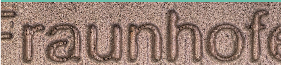
Figure 6: From top to bottom: vertical surface with embossed writing on the reference specimen, shot peened specimen, angled surface with engraved writing on the reference specimen, shot peened specimen
