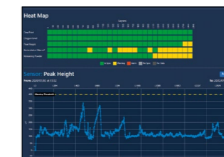
Velo3D build heat map (top) and peak height chart (bottom)
