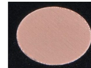
2D layer visualization showing individual laser tracks and fusion defects in high resolution
