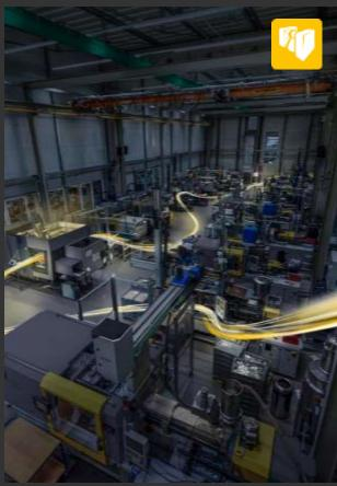
INJECTION MOULDING + MOULD MAKING 28 Injection moulding machines 0.01 to 350 g component weight 150 to 2,200 kn clamping force
